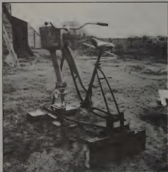
Stripped bicycle wheat grinder. Wheat hopper shown feeding into attrition mill (Corona in this case).
